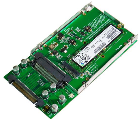
PD425A Adapter with U.2 to M.2 SSD (Samsung SM961)
